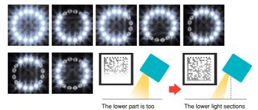
The lower part is too bright so uniformity is not possible and the image is not stable. The lower light sections are turned off, the brightness becomes uniform and a stable reading can be taken.
