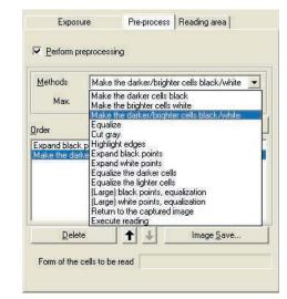
14 types of pre-processing are available. Settings are made by simply selecting from a pull-down menu.
