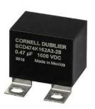
Style SCD offers protection against voltage transients in low to medium current IGBT applications where high dV/dt is encountered. Connect these capacitors from C1 to E2 on a dual IGBT module or from P to N on a six-pack module to eliminate severe voltage transients. Parts ending with Z25 fit IGBTs with 23mm, 25mm and 28mm lead spacing. If you have a preferred lead spacing, please specify.
