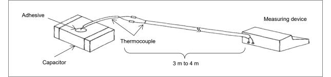
When using a lead-type capacitor with a low mounting heat-resistant temperature, measure the temperature profile of the mounted capacitor by the following method so that the capacitor is soldered at a temperature equal to or lower than the heat-resistant temperature.
