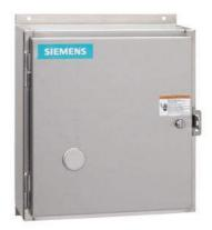
Electrically held lighting contactor, Contactor amp rating 20A, 0 N.C. / 4 N.O. Poles, 220VAC 50HZ/240VAC 60HZ coil, Non-combination type, (no disconnect device), Encl NEMA type 4X 304 S-Steel, Water/dust tight noncorrosive
