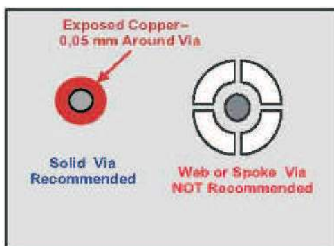
Figure 27. Thermal Via Connection at the Bottom Layer
