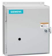
Non-reversing contactor, Size 2 1/2, Three phase full voltage, Contactor amp rating 60A, 3 wire (NO aux included), 208VAC 60Hz coil, Non-combination type, Enclosure NEMA type 12, Dust/drip proof for indoors, Extra-wide enclosure
