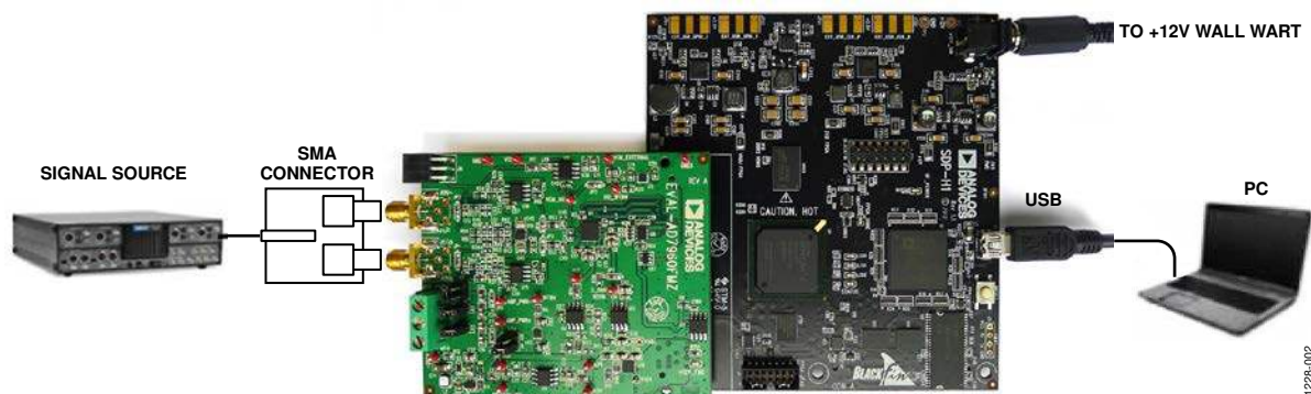
Figure 1. Setting Up the EVAL-AD7960FMCZ
