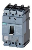
circuit breaker 3VA5 UL frame 125 3-pole, starter protection TM120M, AM, In=10A without overload protection short-circuit protection Ii=3...7 x In cable connection on both sides
