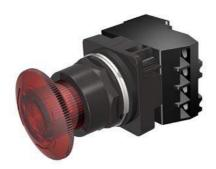
30mm BlackMax, Epoxy Coated Corrosion Resistant Complete Metal Unit Illuminated Twist-to-Release Full Voltage, 120V AC/DC Incandescent Lamp Mushroom Head Cap Small 1.79" (45 mm) Plastic Cap, Red 2 Position Maintained, Twist-to-Release with 1 N.O. - 1 N.C. Heavy Duty Contacts, A600/P600 UL Listed, CSA Certified NEMA 1,3,3R,4,4X,12,13 & Automotive Standards
