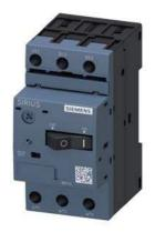
Circuit breaker size S00 for motor protection, CLASS 10 A-release 0.45...0.63 A N-release 8.2 A Screw terminal Standard switching capacity
