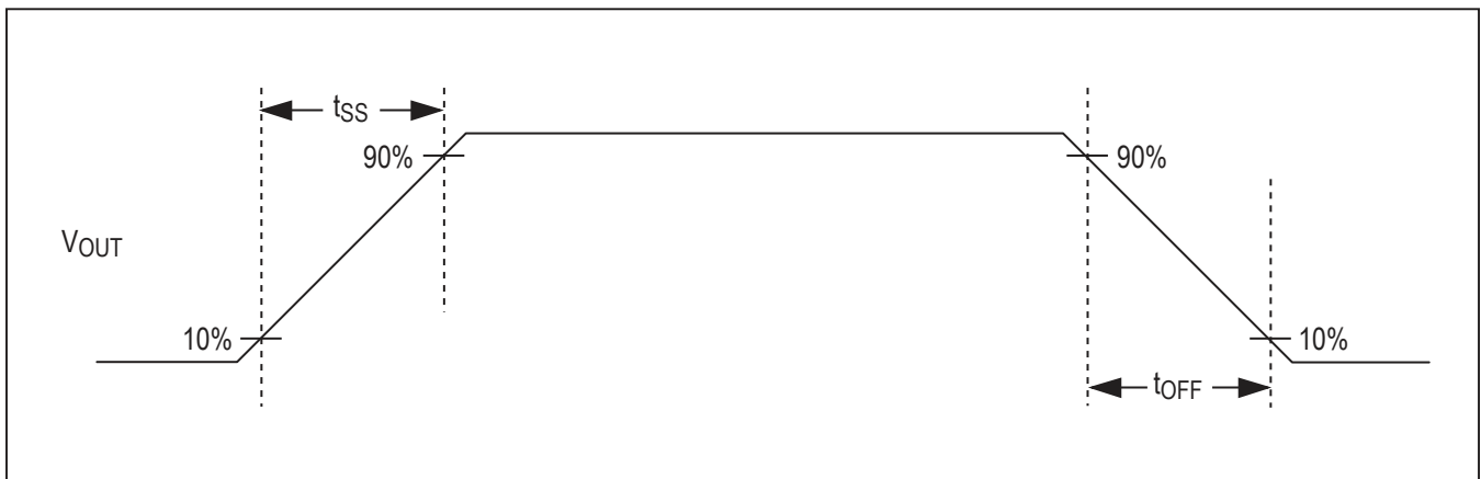
Figure 1. Timing Diagram for Measuring Turn-On Time ( t_{SS} ) and Turn-Off Time ( t_{OFF} ).
