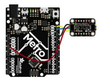
Connect board VIN (red wire) to Arduino 5V if you are running a 5V board Arduino (Uno, etc.). If your board is 3V, connect to that instead.
