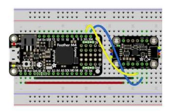
Board 3V to sensor VIN (red wire)
