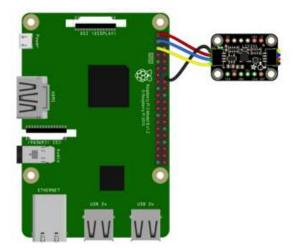
Pi 3V to sensor VCC (red wire)
