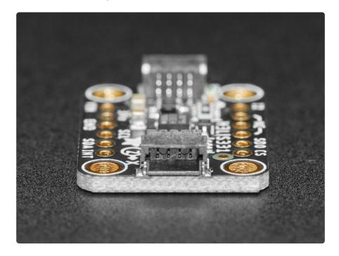
The breakout for the LIS331 family takes one of these little dynamos and puts it on a custom made PCB in the STEMMA QT form factor (), making them easy to interface with. The STEMMA QT connectors () on either side are compatible with the SparkFun Qwiic () I2C connectors. This allows you to make solderless connections between your development board and the LIS331s or to chain them with a wide range of other
