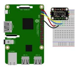
Pi 3V to sensor VCC (red wire)
