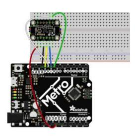
Connect Vin to the power supply, 3V or 5V is fine. Use the same voltage that the microcontroller logic is based off of Connect GND to common power/data ground
