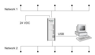
Internally the gateway consists of two separate network interfaces, mounted at the top and bottom end of the gateway respectively, and a translation device handling communication between the interfaces.
