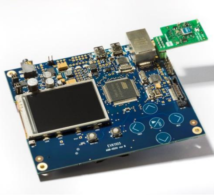
* Photo of the SPB105 connected with the SPI-card interface on the EVK1105. Ready-made downloadable reference designs can be started within minutes and development can start at once.
