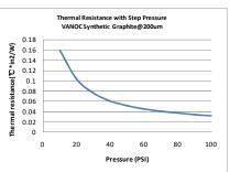
VANOC Synthetic Graphite 200um thick; 1 inch² test sample; Rate of strain = 0.25 mm/min
