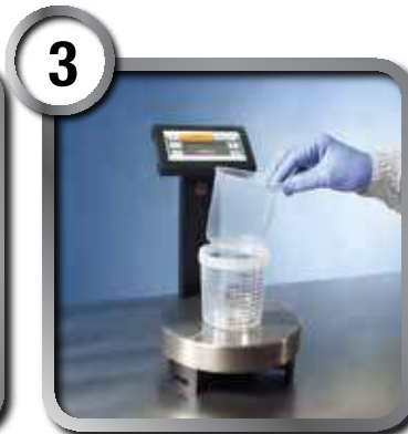
3 Remove liner from wall dispenser and place into 3M™ PPS™ mixing cup. Weigh the paint according to paint manufacturer's guidelines.
