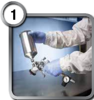
1 Remove existing cup from spray gun.
