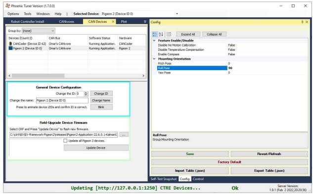
**Note 1:** The Mount Orientation Angles can be specified with Phoenix Tuner or with Phoenix API.
