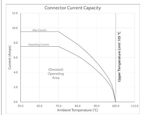
Testing based on IEC 60512-5-2. Max current curve generated with isolated test article under controlled environmental conditions, and does not take into account external factors such as housings, mating cables, or other circuitry. Operating current curve (derated by 20% of maximum values) accounts for external factors, and manufacturing variation.
