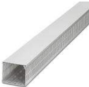
Cable duct, white, comprising upper part and mounting base, width: 30 mm, height: 60 mm, length: 2000 mm
