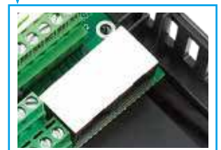
Dual RJ45 communication ports
