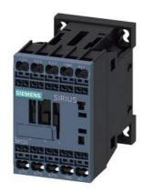
traction contactor, AC-3e/AC-3, 12 A, 5.5 kW / 400 V, 3-pole, 24-34 V DC, 0.7-1.25\* Us, electronic drive, with integrated varistor, auxiliary contacts: 1 NO, spring-loaded terminal, size: S00
