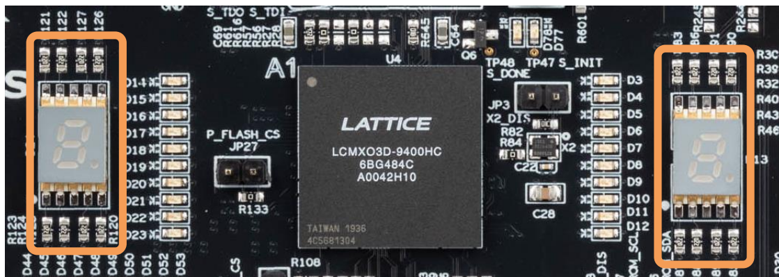
Figure 5.4. Two 7-Segment LEDs for MachXO3D Device
