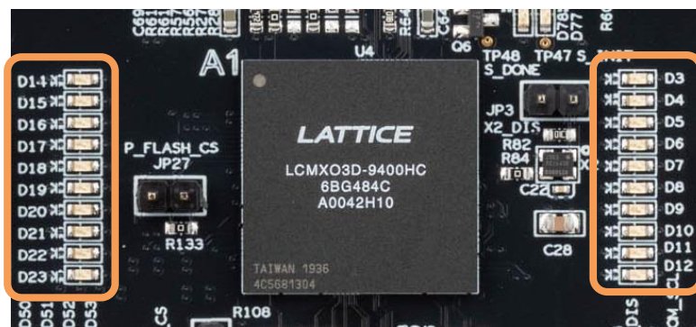
Figure 5.1. 20 Green LEDs for MachXO3D Device
