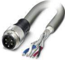
Bus system cable, DeviceNet, 5-position, PVC, Gray RAL 7001, Plug straight 7/8"-16UNF, on Free cable end, Cable length: 5 m
