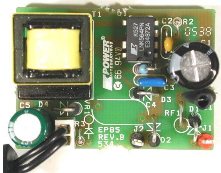
Figure 1 – LNK564 Low Cost Cell Phone Charger Populated Circuit Board Photograph.
