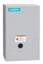
Non-reversing NEMA contactor, Size 2, Three phase full voltage, Contactor amp rating 45A, 3 wire (NO aux included), 380-440/440-480V 50/60Hz coil, Non-combination type, Enclosure NEMA type 1, Indoor general purpose use, Standard width enclosure
