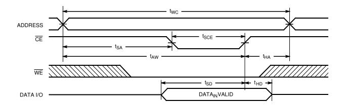
Write Cycle No. 3 ( $\overline{\text{WE}}$  Controlled,  $\overline{\text{OE}}$  LOW)<sup>[11, 16]</sup>
