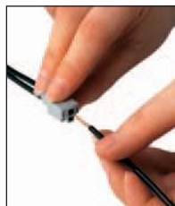
Solid conductor strip (8–9 mm) and connect conductor
