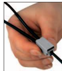
Stranded conductors strip (8–9 mm) conductor, compress terminal and insert conductor
