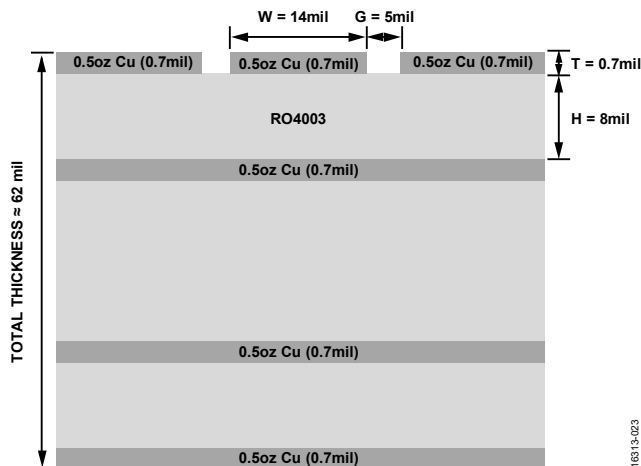
Figure 23. Evaluation Board (Cross Sectional View)
