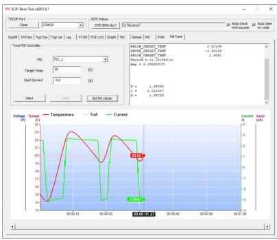
Set a suitable target temperature click the START button the temperature can be observed cycling twice, in the graph window, the PID information will appear in the output window Click Set Pid Values to set the PID
