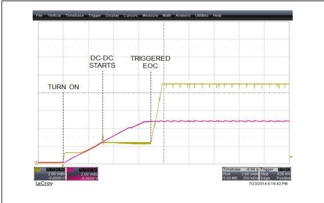
Figure 13. Buck-boost startup ( I_{IN} = 5\ \mu\text{A} )
