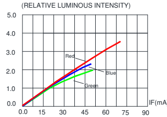
FIG.2 RELATIVE LUMINOUS INTENSITY VS. FORWARD CURRENT
