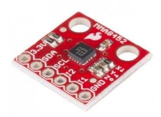
The MMA8452Q is just a solid 3-axis accelerometer. It supports three, selectable sensing ranges: ± 2g, 4g, or 8g. It sports features like orientation detection, single and double-tap sensing, and low power modes. It's a
