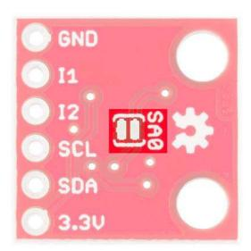
By default the jumper is open, which will pull the SA0 pin high (there's a resistor on the top side of the board to help accomplish that task). If you close the jumper, by applying a small solder blob to connect both pads together, SA0 will be pulled to ground.
