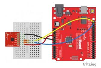
We simply have to supply the accelerometer with power (3.3V and GND), then hookup the SCL and SDA lines between devices. A couple of  $330\Omega$  resistors in series on each I<sup>2</sup>C line will help to perform some simple level shifting. If you want more advanced level shifting...
