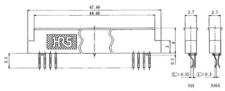
• Recommended board thickness: 0.4 to 0.5mm
