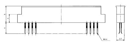
• Recommended board thickness: 0.4 to 0.5mm
