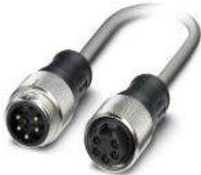
Bus system cable, DeviceNet, 5-position, PUR halogen-free, Gray RAL 7001, Plug straight 7/8"-16UNF, on Socket straight 7/8"-16UNF, Cable length: 20 m
