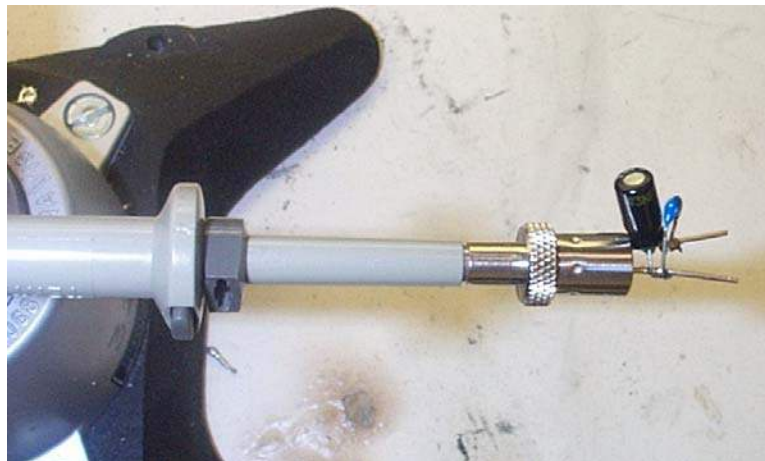
Figure 22 - Oscilloscope Probe with Probe Master 5125BA BNC Adapter (Modified with Wires for Probe Ground for Ripple Measurement, and Two Parallel Decoupling Capacitors Added).
