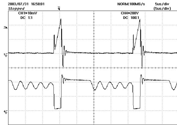
Figure 13 - 265 VAC, Full Load. Upper: I_{DRAIN} , 0.1 A / div. Lower: V_{DRAIN} , 200 V / div, 5 \mu s / div.
