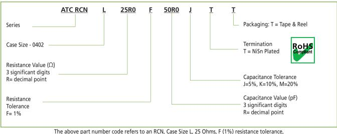
50 pF, J (5%) capacitance tolerance, T termination, with tape and reel packaging
