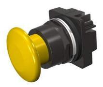
30mm BlackMax, Epoxy Coated Corrosion Resistant Metal Operator, Round Push-Pull Operator Non-Illuminated Mushroom Head Cap Small 1 3/4" (44.5 mm) Plastic, Yellow 3 Position Pull-Momentary/Push-Maintained UL Listed, CSA Certified NEMA 1,3,3R,4,4X,12,13 & Automotive Standards
