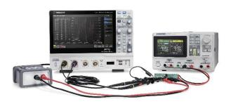
The oscilloscope can control the built-in waveform generator or a stand-alone SIGLENT generator, to scan the amplitude and phase-frequency response of the DUT, and display the data as a Bode Plot. This makes it possible to replace expensive network analyzers in some applications
