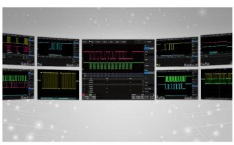
Display the decoded characters through the events list. Bus protocol information can be quickly and intuitively displayed in tabular form. I<sup>2</sup>C, SPI, UART, CAN, LIN, CAN FD, FlexRay, I<sup>2</sup>S, MIL-STD-1553B, SENT, and Manchester are supported
