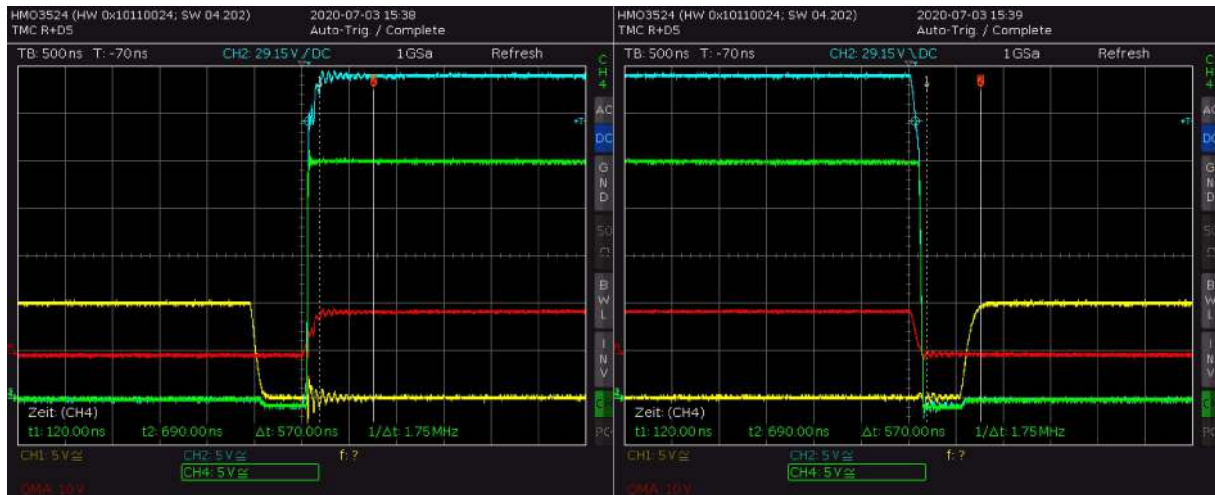
Figure 6: Ringing of output (green) and gate voltages (yellow, blue) with DRV_STRONG=0
