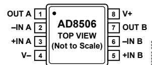
Figure 3. 8-Lead MSOP (RM-8)
