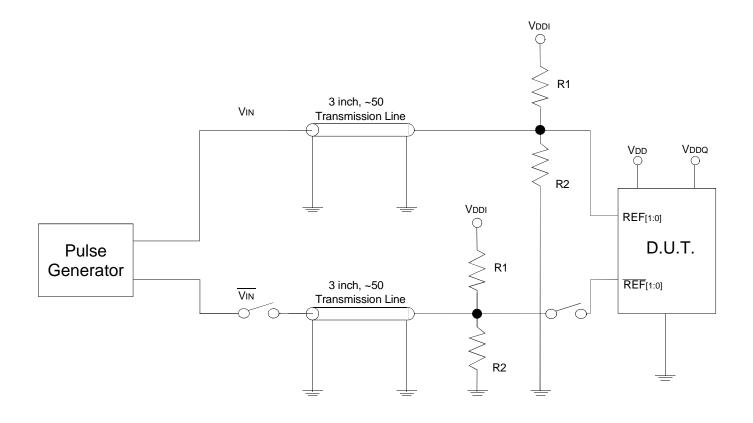
Test Circuit for Differential Input<sup>(1)</sup>
