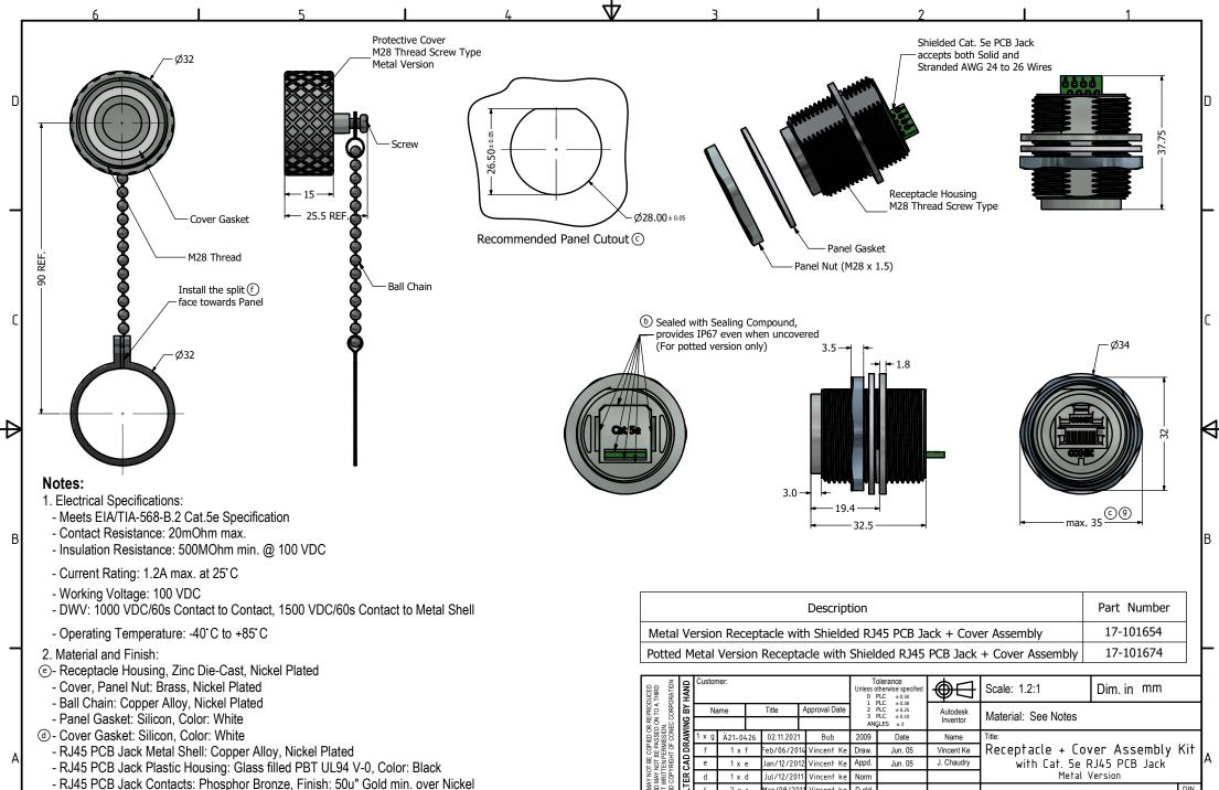
3. Connector can be front or rear mounted to a maximum panel thickness of 3.2mm.
