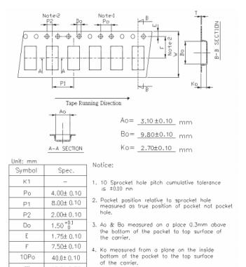
Carrier camber shall be not than 1mm per 100mm through a length of 250mm.
