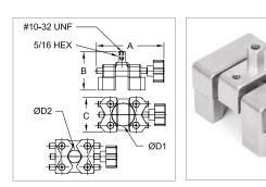
\* Reverse the jaws to switch from ØD1 to ØD2 Includes a #10-32 M/M stud with jam nuts
