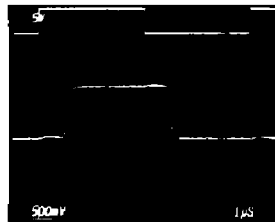
MUX-24 SMALL-SIGNAL SWITCHING WITH FILTERING
