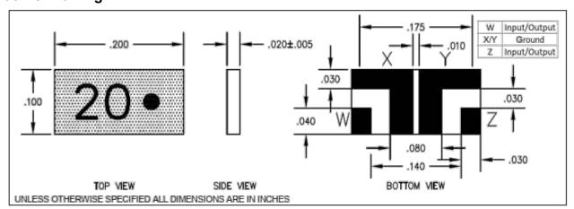
Tolerance is  $\pm 0.010$ ", unless otherwise specified. Designed to meet or exceed applicable portions of MIL-E-5400. **All dimensions in inches.**
