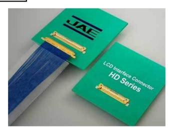
JAE has developed the HD Series of connectors (HD1: 40 pos. HD2: 30 pos.) for notebook PC LCD interface applications. The HD Series connectors are compatible with LVDS transmission and LED backlight as standardized in the VESA® 16:9 Wide Notebook Panel Standard, and are licensed products for the Dai-ichi Seiko Co., Ltd. (I-PEX) CABLINE®-VS.
