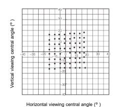
(2) Each pixel's viewing angle (half angle)
