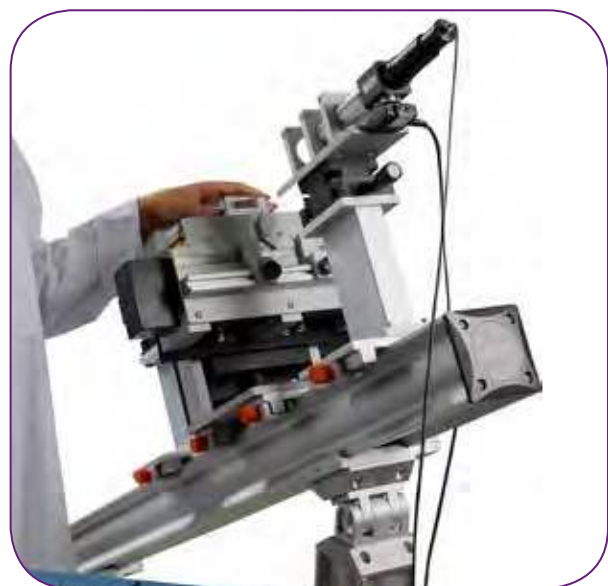
Fig. 5 Measuring station for determining geometric parameters of cylindrical lenses out of X95 components built by OEG GmbH.
