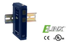
The Elinx™ EIRSP1 Industrial Ethernet Surge Protector is designed to protect all eight lines used in a standard CAT5e Ethernet cable. It is compatible with 10/100BaseT networks and 802.11af (Modes A & B) Power Over Ethernet. Mode A applies power to the data pairs, pins 1/2 and 3/6. Mode B applies power to the unused pairs, pins 4/5 and 7/8.
